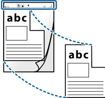
2. Load the Carrier Sheet into the left side of input slot with the top edge facing into the scanner. Slide the Carrier Sheet into the input slot until it meets resistance.
