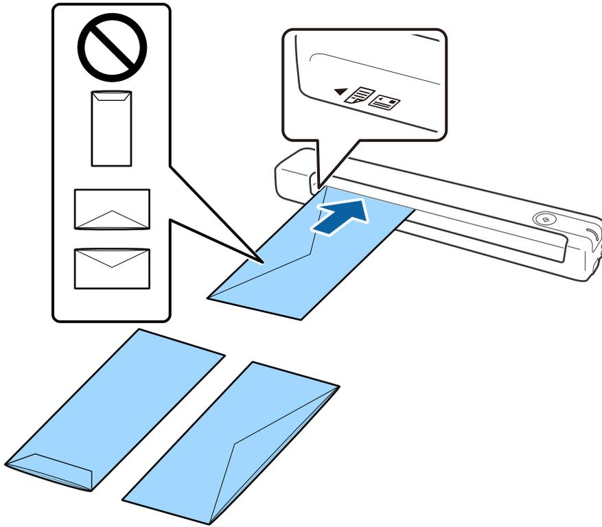
The envelope shown in the illustration has the opened edge (flap side) facing up, but you can also load envelopes into the scanner with the opened edge (flap side) facing down.
