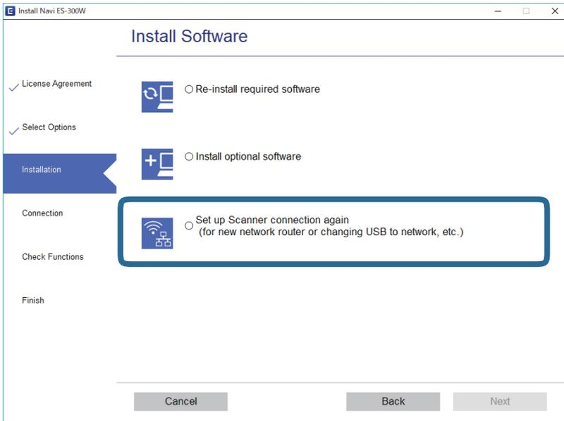
Select **Set up Scanner connection again (for new network router or changing USB to network, etc.)** on the Install Software screen, and then click **Next**. Follow the on-screen instructions.
