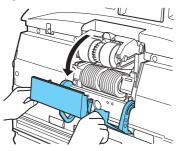
3 Pull the roller lock lever down.
