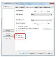
• Select the [Erase Dot] check box to automatically remove isolated black dots (3 x 3 dot size) from white backgrounds (or white dots from black backgrounds).
