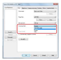
If the scanning side is set to [Skip blank page], the images of blank pages are deleted when images are saved.
