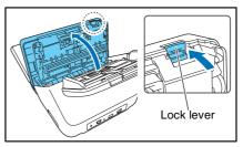
Pull out the jammed document in the direction that seems the easiest to remove it.
