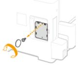
**2** Open the ROM cover, and remove it in the direction indicated by the arrow.
