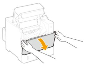
**4** Remove the envelope feeder cover.
