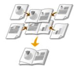
You can print two pages of a document on both sides of paper and then fold your printed pages in half to make a booklet. The printer driver controls the print order in such a way that the page numbers are correctly arranged.
