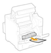
**6** Replace the envelope feeder back in place.
