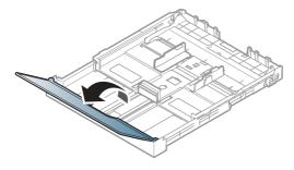
3 Squeeze and the paper width guide and paper length lever to locate them in the correct paper size slot marked at the bottom of the tray to adjust to the size.
