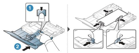
For paper longer than A4-sized(like 'Legal'), press and unlatch the guide lock in the tray, pull the tray out manually. Then adjust the paper length guide and paper width guide.
